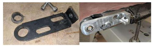
can be tweaked to drift right or left. Also the bearings have been replaced on the feed side and one of the bearing brackets was remade. Hopefully, this time users will use reasonable tightening forces and pay full attention to the adjustments they are making. Then no further repairs will be required. Remember, this is a finishing tool, not a stock removal tool.
